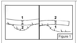
First cut a force relief groove from the tight side (1), and then cut it into the loose side (2).
