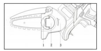
**NOTE:** The top and bottom of the guide bar are symmetrical, and the bar may be mounted with the printing facing up or down. Flipping the guide bar each time the chain is sharpened or changed will help reduce uneven wear and improve its service life.
