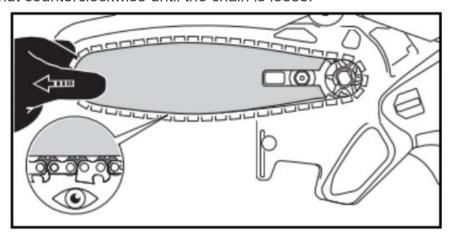
e) Pull the guide bar to tighten the chain.
